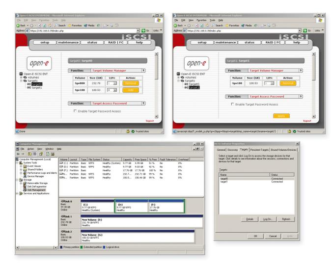
A striking advantage: Within an operating system - here Windows XP - iSCSI displays storage space on the network as a local drive, and also allows it to be managed like one.
