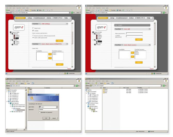
The screen shots show user authorization settings on the web-based graphic user interface of Open-E NAS and secure access to NAS storage from a Windows client.
