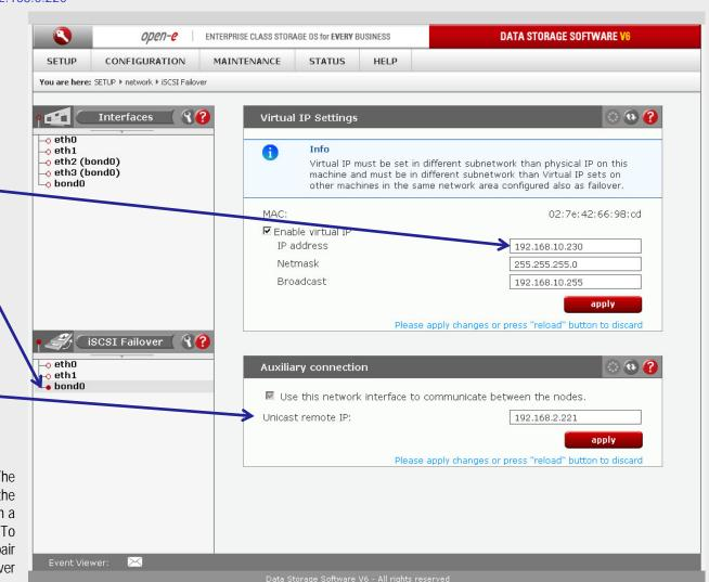
7. Configure Virtual IP and Auxillary connection
