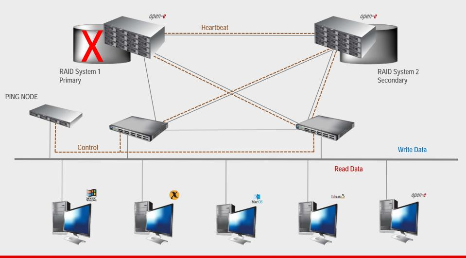
• After switching, the replicated volume is available on System 2 (secondary)
