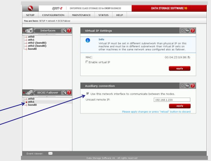
Now, select the <u>eth1</u> within <u>iSCSI Failover</u>. In the Auxiliary connection function check box Use this network interface to communicate between the nodes next enter IP address for Unicast remote IP and click the apply button.
