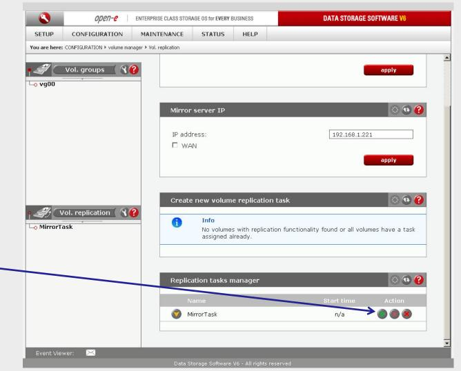
Now, in the **Replication task** manager function, click on button under to start the Replication task on the Primary node
